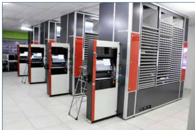
Figure 2: The Pharmacy Dispensing Unit: robotic dispensing system
